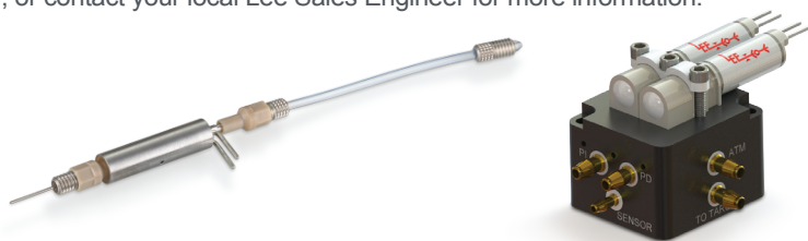
Left: A VHS Series dispense valve shown with an interchangeable threaded nozzle on the outlet and MINSTAC® fitting threaded into the inlet. Right: The compact LFMX0534570B Reversible Flow Manifold (29 x 25 x 19 mm) comes with two LHD Series valves and is plumbed to enable switching between vacuum and pressure.
