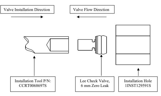
2. The installation tool (P/N: CCRT0068697S) is used to simply press the valve into a plastic installation hole until the valve is at a minimum flush with the top of the installation hole.
