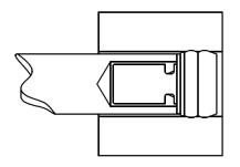
3. The series of smoothly curved lands of the Lee Check Valve, 6 mm Zero Leak, Press-In seals and retains the product in the plastic installation hole.
