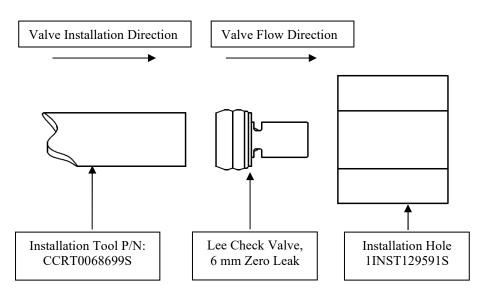
2. The installation tool (P/N: CCRT0068699S) is used to simply press the valve into a plastic installation hole until the valve is at a minimum flush with the top of the installation hole.
