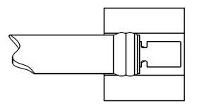
3. The series of smoothly curved lands of the Lee Check Valve, 6 mm Zero Leak, Press-In seals and retains the product in the plastic installation hole.
