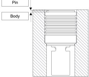
3. When the installation tool is retracted, the installed product can be inspected by measuring the depth of the top of the pin relative to the top of the body. The distance should be less than 0.25 mm. The pin should not be pushed below flush of the body.
