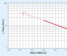
The LT Series Disc Pump has no prevalent sudden failure mode. Instead, the operational wear processes in the pump eventually contribute to a gradual reduction in peak pressure capacity and efficiency. The Lee Company defines a point in time, t1, at which these wear processes start to affect pump performance. In many cases, the pump continues to meet application requirements beyond t<sub>1</sub>. t<sub>1</sub> varies with drive power (amongst other operational parameters).
