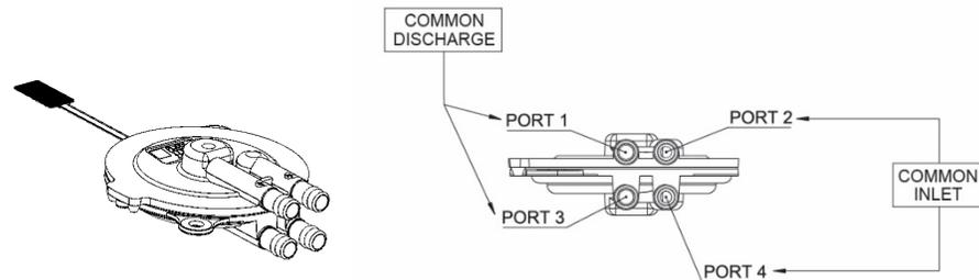
Figure 11. BL/XP/LT Series, parallel configuration pumps - port numbering
