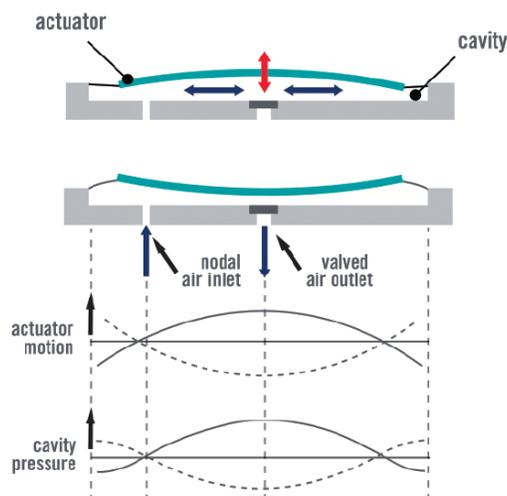
Figure 1. A schematic of the disc pump
