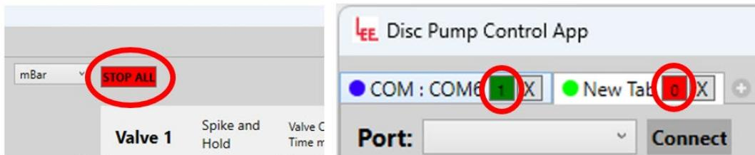
Figure 46. Stop all button (left) and pump on/off control from tab title (right).
