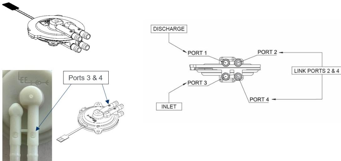
Figure 6. BL/XP/LT Series, series configuration pumps - port numbering
