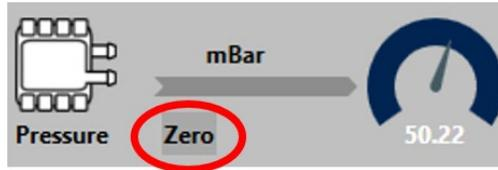
Figure 36. Zeroing the pressure sensor
