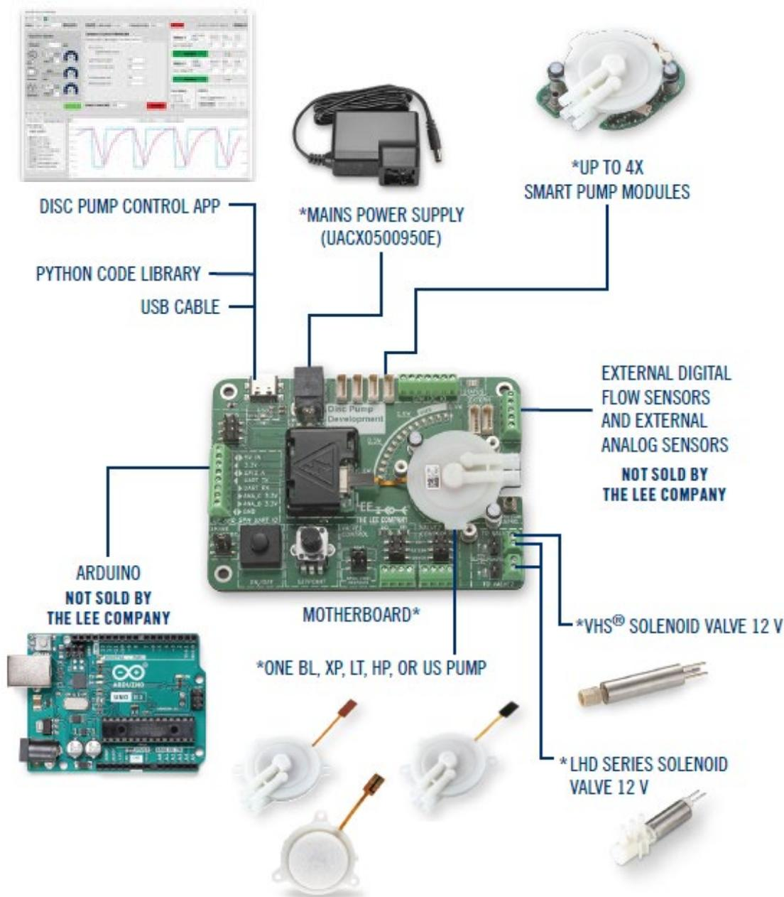
Figure 3. Disc Pump Development Kit connectivity for disc pumps/modules, solenoid valves, external sensors and microprocessors.
