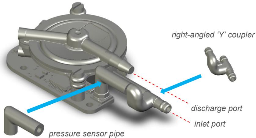
Figure 20. Connecting an HP Series pump for vacuum pressure regulation with the prototype connectors supplied with the optional SPM Prototype Pneumatic Adapter Kit (UACX0500600H)
