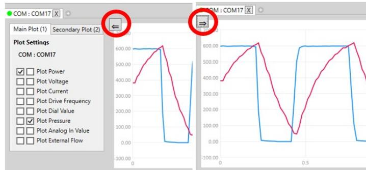
Figure 40 Showing and hiding the plot settings
