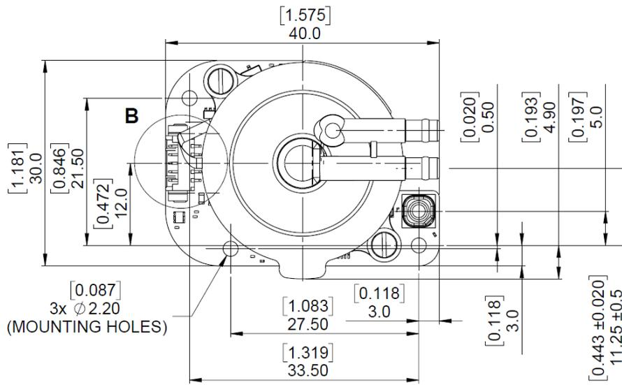
Figure 4: SPM Geometry. Dimensions in mm [inches]
