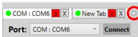
Figure 42. Adding and removing additional pump control tabs.
