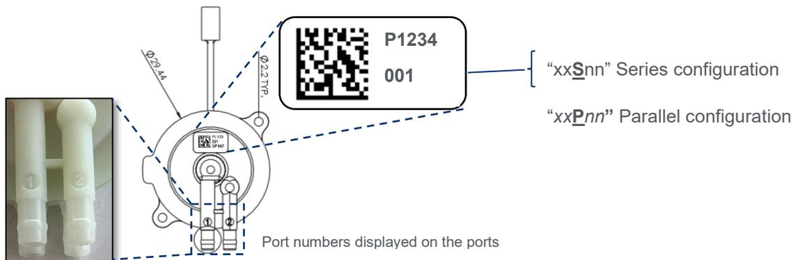
Figure 5. Pump labelling to distinguish between series and parallel configuration pumps
