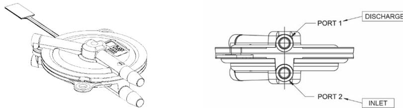
Figure 16. HP Series pumps - port numbering
