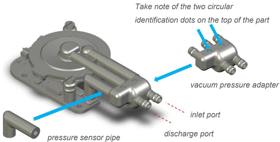
Figure 15. Connecting a parallel configuration pump for vacuum pressure regulation with the prototype connectors supplied with the optional SPM Prototype Pneumatic Adapter Kit (UACX0500600H)
