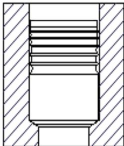
3. When the installation tool is retracted, the pin should be flush to within 0.25mm above flush of the insert body
