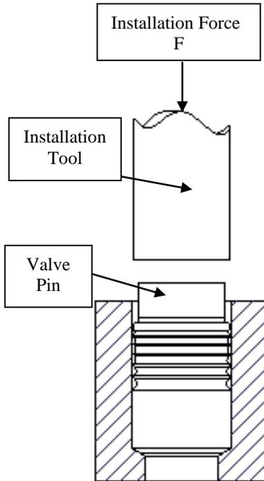
1. The Lee Check Valve, 558 Series, Reverse, Insert, Screened product is inserted into the installation hole with the pin end up as shown.
