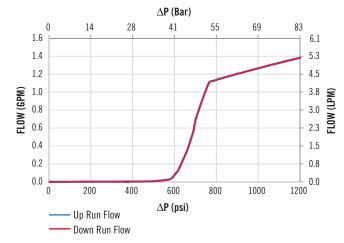
Typical Flow Curve for 40 Bar Valve
