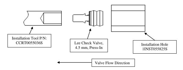
The installation tool (P/N: CCRT0055036S) is used to simply press the valve into a
