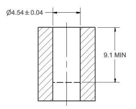
DIMENSIONS IN MILLIMETERS Note: Draft angle to fall within diameter tolerance Refer to Lee Drawing No. 1INST055825S
