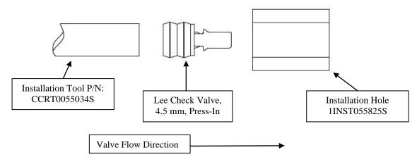
2. The installation tool (P/N: CCRT0055034S) is used to simply press the valve into a plastic installation hole until the valve is at a minimum flush with the top of the installation hole.
