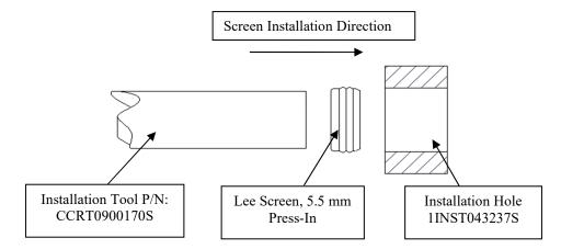
2. The installation tool (P/N: CCRT0900170S) is used to simply press the Screen into a plastic installation hole until the product is at a minimum flush with the top of the installation hole.
